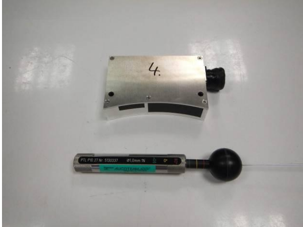
Picture 1 Sensor head MHAP XXX specimen with rigid steel wire (Ø 1 mm, 1 N) during contact protection test IP6X
