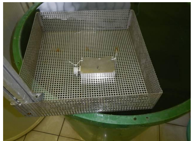
Picture 5 Sensor head MHAP XXX specimen with portable compact tester insulation test after the immersion substitute test IP6X before the immersion substitute test IP6X
