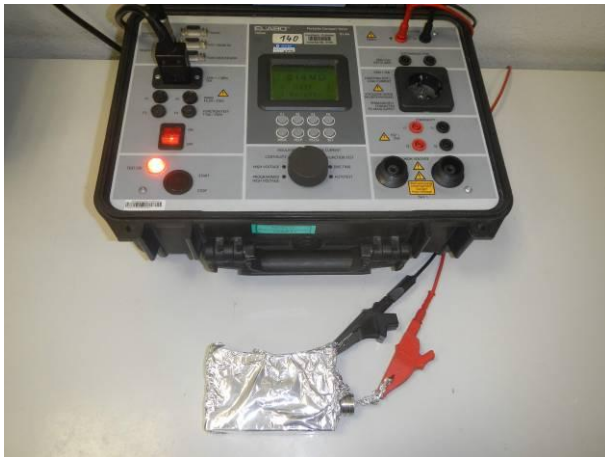
Picture 3 Sensor head MHAP XXX specimen with portable compact tester insulation test before immersion substitute test IP6X
