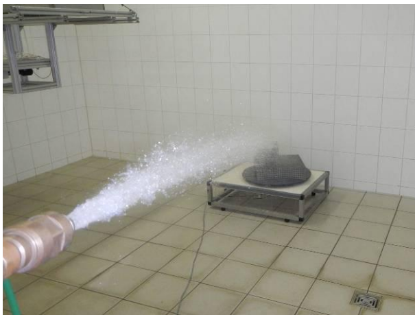
Picture 9 Sensor head MHP XXX on the turn table with water from the spray nozzle during the water jet test IPX6
