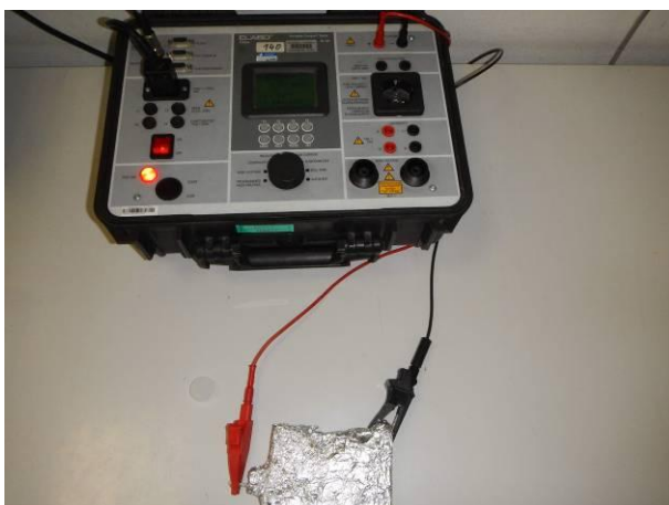
Picture 11 Sensor head MHP XXX specimen with portable compact tester insulation test after the water jet test IPX6
