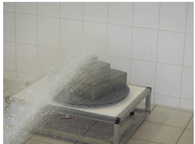
Picture 10 Sensor head MHP XXX on the turn table with water from the spray nozzle during the water jet test IPX6
