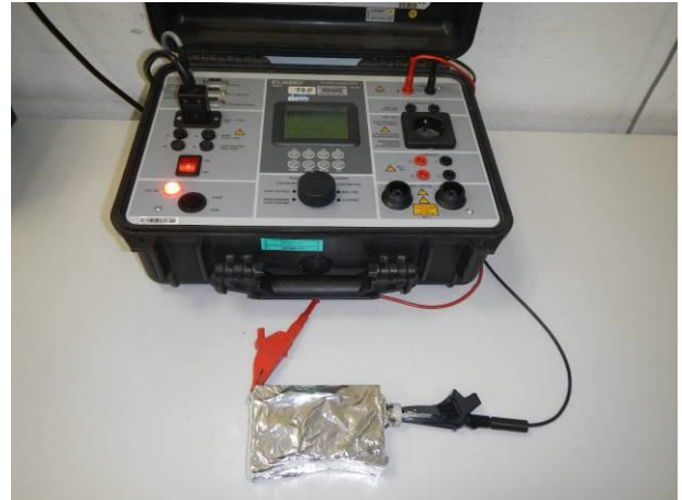
Picture 8 Sensor head MHP XXX specimen with portable compact tester insulation test after the water immersion test IPX7
