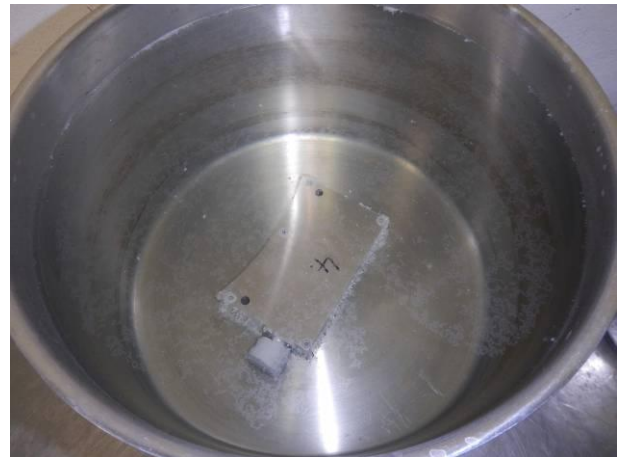
Picture 4 Sensor head MHAP XXX specimen in the dipping basin 200 mm during the immersion substitute test IP6X
