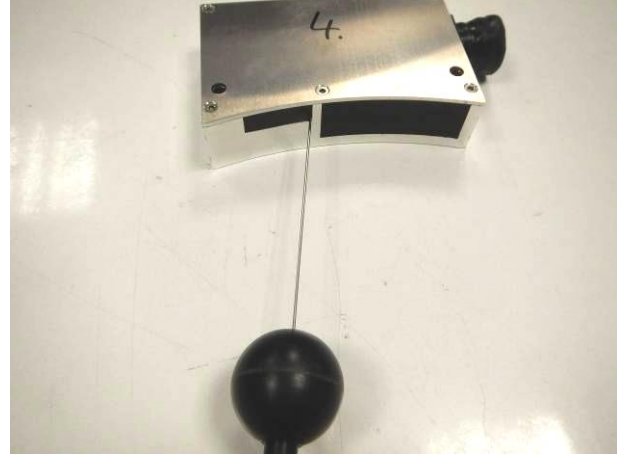
Picture 2 Sensor head MHAP XXX specimen with rigid steel wire (Ø 1 mm, 1 N) during contact protection test IP6X
