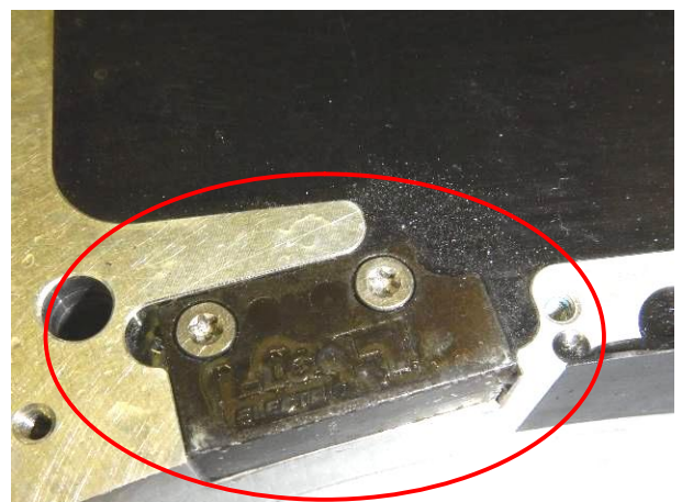
Picture 12 Sensor head MHP XXX traces of water on the sealing compound inside after the protection tests IP67 and IPX6
