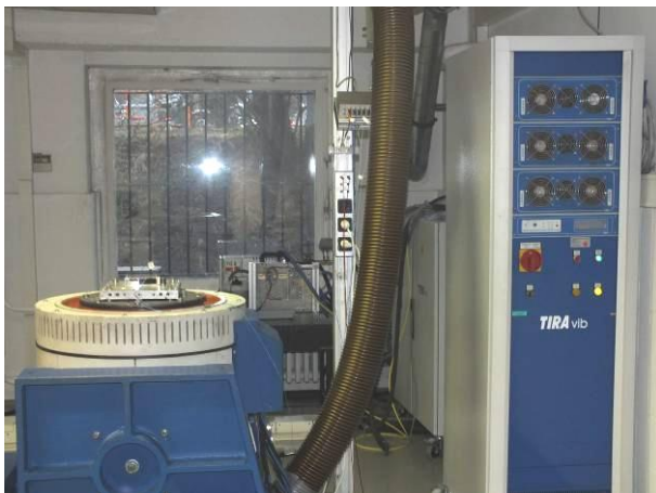
picture 5 Sensor Head MHAP specimen on the vibration test device during vibration test in Z-axis
