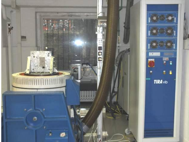
picture 1 Sensor Head MHAP on the vibration test device during vibration test in X-axis
