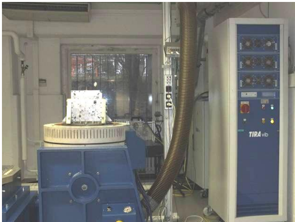
picture 3 Sensor Head MHAP specimens on the vibration test device during vibration test in Y-axis
