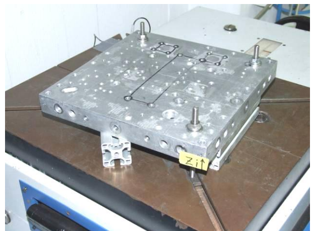
picture 12 Sensor Head MHAP on the shock table with acceleration sensor during shock test in Z-axis, negative direction
