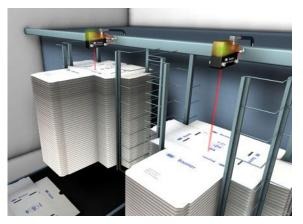
*Fig. 2: Using photoelectric sensors to measure stack height in the printing or packaging industry*
