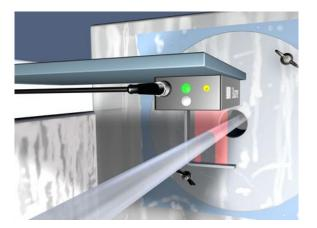
Fig. 4: Using line sensors to measure wire and cable widths for quality control purposes
