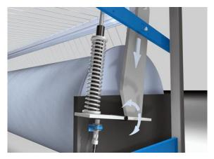
Fig. 3: Using measuring inductive sensors to control thread tension on an automated loom
