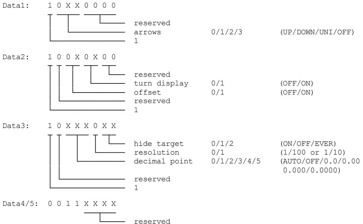
**Important:** Only bits marked ‘X’ may be altered. The fix values „1“ and „0“ must not be altered since thereby a control token (tokens < 20h) might be created what is not allowed in ASCII protocol.
