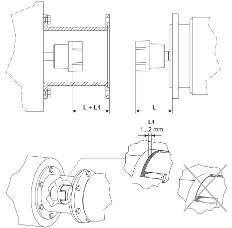
III. 8: Correct assembly of a claw coupling
