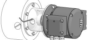
III. 4: Installing encoder, mounting device and coupling
