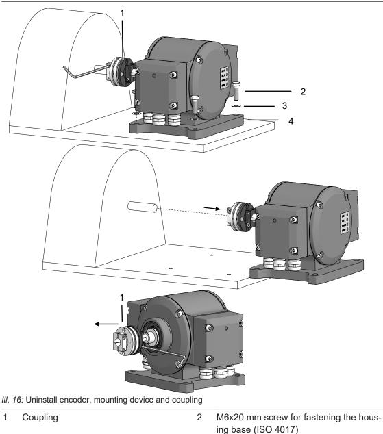
3 Washer B6 for fastening the housing 4 Housing base base (DIN 137)
