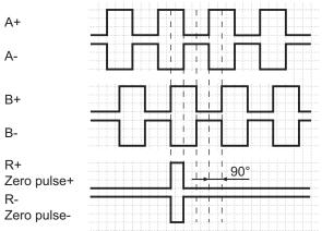
*III.* 12: Output signals with positive direction of rotation (zero pulse R+ and R- are only available at additional output II)
