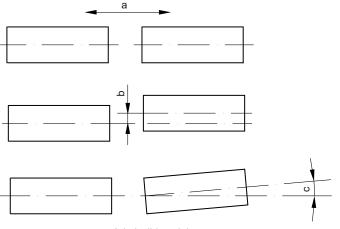
a = Admissible axial movementb = Admissible parallel misalignmentc = Admissible angular error
