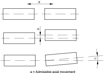
a = Admissible axial movement b = Admissible parallel misalignment c = Admissible angular error
