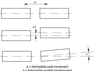
a = Admissible axial movement b = Admissible parallel misalignment c = Admissible angular error
