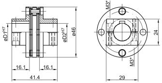
\* Maximum tightening torque: Mt = 1 Nm (plastic side) Mt = 1.3 ±10 % Nm (metal side)
