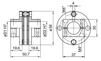
\* Max. tightening torque: Mt = 1.5 Nm (plastic side) Mt = 2-3 Nm (metal side)
