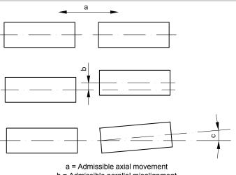
b = Admissible parallel misalignment c = Admissible angular error
