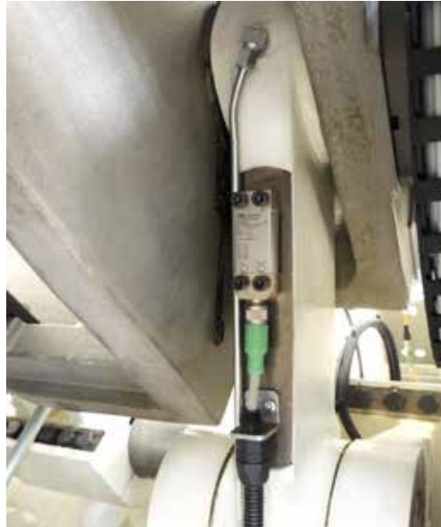
The Baumer DSRT strain sensor on the toggle lever reliably monitors the clamping force of the RDM-K machines.
