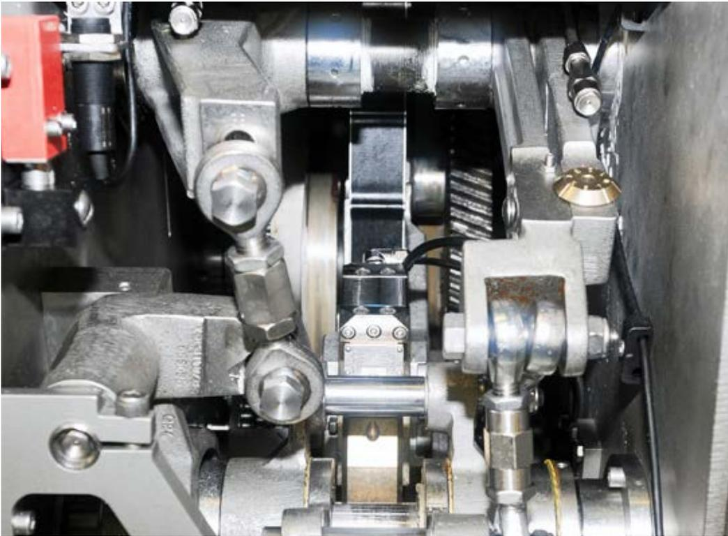
The DST55R strain sensors do not have to be adapted to the machine design in a time-consuming process, but can easily be bolted onto the ideal place – here on the plunger.
