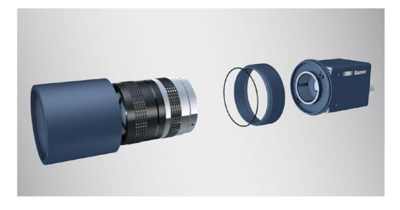
Thanks to the patented modular lens protection system, available with M47 or M62 threads, cameras and lenses of various lengths and diameters can be protected quickly and flexibly with a variable number of extension rings, ensuring compliance with protection classes IP 54, IP 65, and IP 67.
