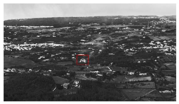
Fig. 4: While still in the monitoring tower, a feature-based algorithm and AI in Sintra evaluate the image data from the cameras and, in the case of suspicion, alert an operator within approx. three minutes, who then decides on the further course of action.
