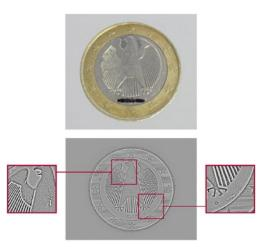
Reliable detection of the finest irregularities in structure and shape even on reflective, glossy or colored surfaces.
