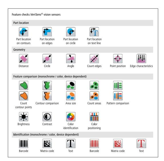
Baumer VeriSens® vision sensors offer 30 tools for up to 32 feature checks in one single inspection task.
