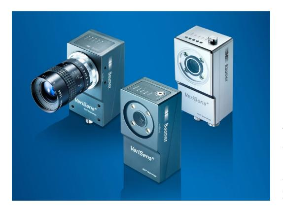
Vision sensors are compact image processing systems in the shape of a sensor. The industry-capable housing integrates what it takes to master an inspection task: C-mount interface with flash controller (left), IP 69K-rated protective housing (right), with integrated optics and white illumination (front).
