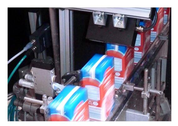
Throughout all industries, vision sensors master vision-based inspection tasks, here in quality control at beverage packaging which is checked upon presence and position of the drinking straw.
