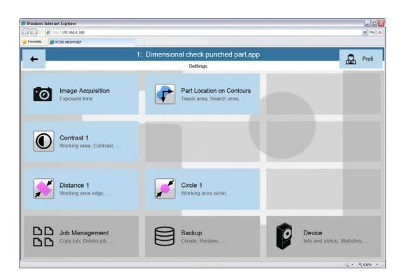
Live shots of the running process provided by the configurable web interface can be accessed any time. Task-specific parameterization is performed directly in the machine browser.
