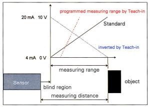
Figure 3: Programmable characteristic probe line
