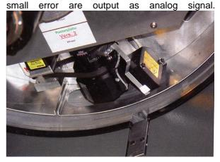
Figure 2: Laser light meter
