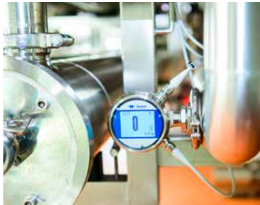
By optimizing the CIP cleaning process, up to 100,000 liters of water can be saved per day thanks to the Baumer conductivity sensor CombiLyz AFI.
