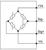
Note on electromagnetic compatibility: Shielded supply cable is recommended. Ground the cable shield on both sides over a large surface and ensure potential equalization. Disconnect the system from power prior to connecting the device.
