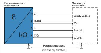
Output signal: IO-Link, parameterizable Operating voltage range: +Vs = 18 to 30 VDC
