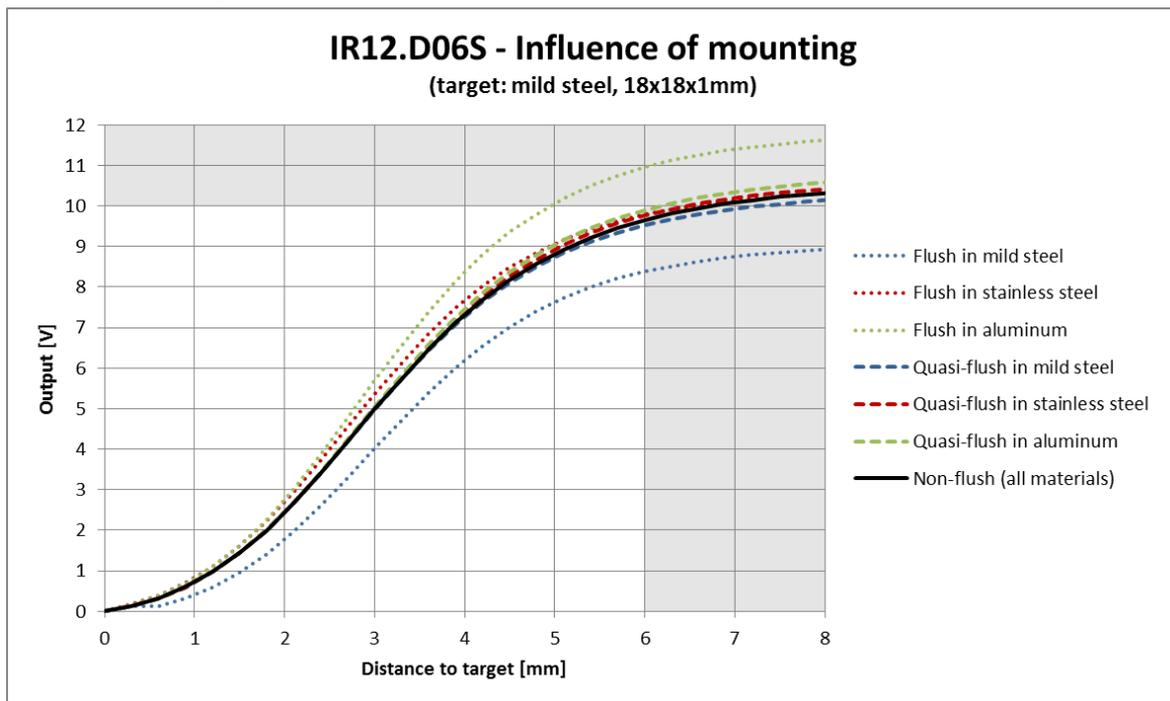
Diagram IR12-D06S sensors: Sensor output (typical values) influenced by different mounting situations (material and position). The mounting material has almost no influence on the output curve for non-flush mounting – as well as quasi-flush mounting and sensing distances up to 50% of  $S_d$ . Nonferrous materials, such as brass or copper, show similar results as aluminum.
