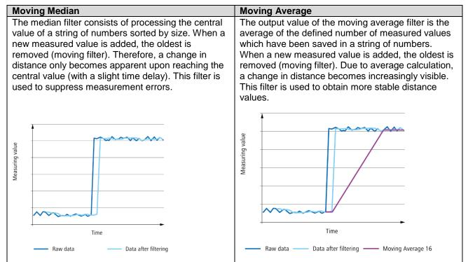
The higher the number of measured values per filter, the longer the response time of the sensor. This means that a change in distance only becomes fully visible for the output after a delay.
