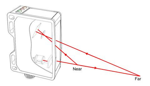
This distance sensor is based on the triangulation principle, which in turn is based on angulation. To carry out the distance measurement, the sensor transmits a light beam, in this case a laser beam, to the object. The light reflected from the object strikes a receiver line inside the sensor at a special angle, depending on the distance. With the help of triangulation, the distance to the object can be determined based on the relationship between the transmission and reception angle.
