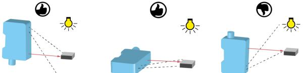
When mounting optical sensors, it is important to ensure that there is no strong ambient light in the area of detection of the receiver.
