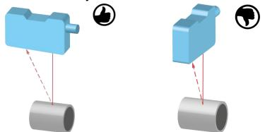
With round, shiny surfaces, the sensor should be aligned in the same axis as the round object in order to avoid reflections.
