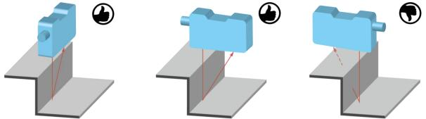
If measurements are carried out directly beside steps/edges, make sure that the reception beam is not covered by the step/edge. The same applies when the depth of holes and cracks is measured.
