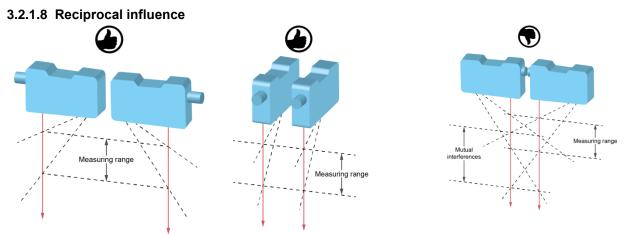
If several optical sensors are used, they may mutually influence one another. During mounting, ensure that only the sensor's own laser spot is in the detection range of the receiver. Up to a measuring range of 600 mm, the sensors can be lined up in a row without them influencing each other (picture in the middle). If the mutual interference cannot be avoided through mounting, the sensors can be operated asynchronously using the Sync-in input, see section "Trigger Mode".
