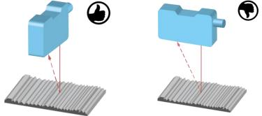
Particularly with shiny objects, for example turned parts, ground surfaces, extruded surfaces and the like, the mounting position affects the measuring result.
