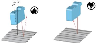
With shiny surfaces, it is important to ensure that the direct reflection does not strike the receiver. This can be prevented by tilting the sensor slightly. To check this, place a sheet of white paper on the disc of the receiver; the direct reflection can then be seen clearly.
