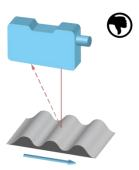
If the contour of an object is measured, it is important to ensure that the object moves at right angles to the sensor, to avoid shadowing and reflections on the receiver.
