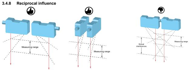
If several optical sensors are used, they may mutually influence one another. During installation, ensure that only the sensor's own laser spot is in the detection range of the receiver. Up to a measuring range of 600 mm, the sensors can be lined up in a row without them influencing each other (picture in the middle). If the mutual interference cannot be avoided through installation, the sensors can be operated asynchronously using the Sync-In input, see chapter TRIGGER MODE.
