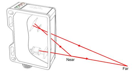
In the triangulation principle, the sensor transmits a light point or light beam to the object to be measured, and the reflected light strikes a receiver line in the sensor at a special angle. Depending on the distance, the angle of incidence changes and thus so does the position of the light spot or light beam on the receiver. The microcontroller allows the suppression of interfering reflections, thus providing reliable data even on critical surfaces.
