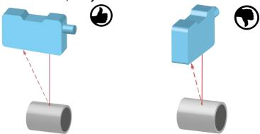
With round, shiny surfaces, the sensor should be aligned in the same axis as the round object in order to avoid reflections.
