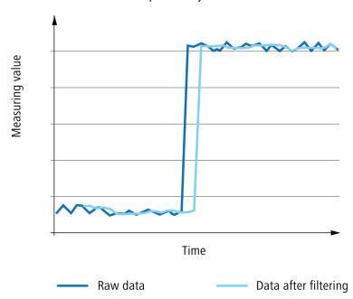
This diagram shows the effects of the median (number of measured values 5). The filter is used to suppress measurement errors. The output only changes after a defined number of measured values (number of measured values/2). The measuring frequency is not affected by this filter, but the response time is.
