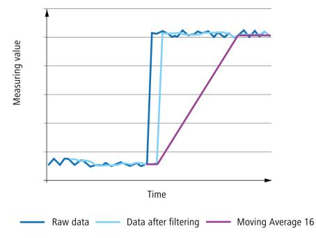
As shown in the diagram, the moving average evens out the output value. In contrast to the median filter, it is possible that with the moving average, the displayed measured values were never measured as such. The measuring frequency is not affected by this filter, but the response time is.
