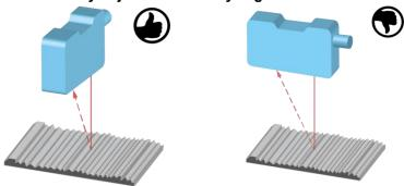
Particularly with shiny objects, for example turned parts, ground surfaces, extruded surfaces and the like, the installation position affects the measuring result.
