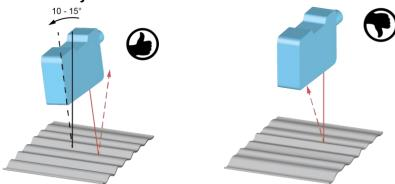
With shiny surfaces, it is important to ensure that the direct reflection does not strike the receiver. This can be prevented by tilting the sensor slightly. To check this, place a sheet of white paper on the disc of the receiver; the direct reflection can then be seen clearly.
