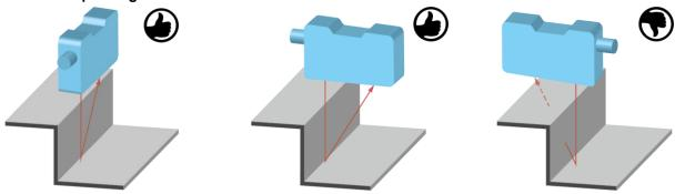
If measurements are carried out directly beside steps/edges, make sure that the reception beam is not covered by the step/edge. The same applies when the depth of holes and cracks is measured.
