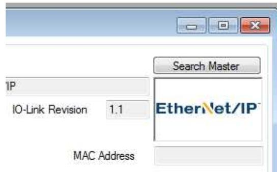
A list with the found IO-Link masters will show up. The master to be taken over will be selected with a double click. The right mouse button enables further functions such as changing the network settings and blinking.
