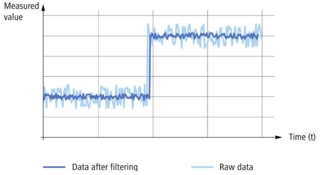
Figure 1: Signal processing moving average filter
