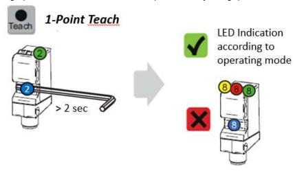
Figure 27: Teach-In procedure Xpress by using qTeach
