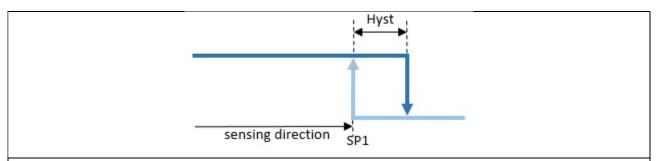
Figure 11 Hysteresis is the difference between switch point and reset point
