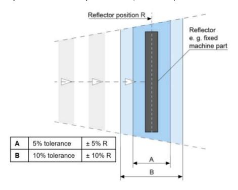
Figure 18: Reflector tolerance reflective barrier
