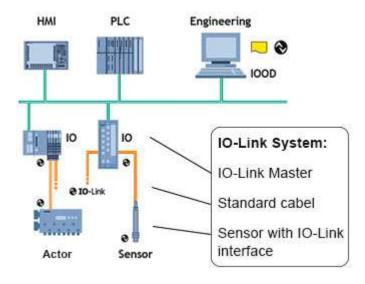
Figure 1 Example of a system architecture using IO-Link
