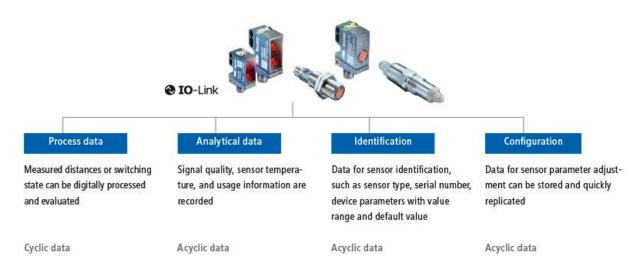
Figure 2 Different IO Link data streams
