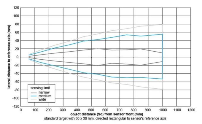
Figure 2: Sonic cone Input Mode adjustment
