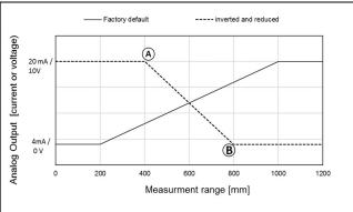
**Figure 33** Reduced range of the analog output value for improved accuracy (analog value increased with distance)
