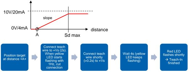
Teach procedure: 1-point teach analog (the target is close and moves away from sensor)
